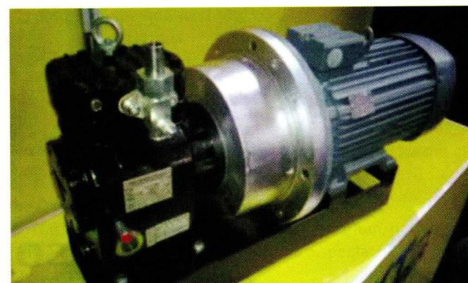
Photo 13: 7 kW ammonia reciprocating compressor
